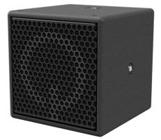
MODEL type filter power handling program power impedance sensitivity program SPL 1m peak SPL 1m frequency range dispersion weight size (wxhxd) **T4** 4"/1" coaxial 1-channel DSP control 100W 200W 8 Ohms 91dBWm 114dB 120dB 100Hz-18kHz 100<sup>®</sup> conical 2,5 kg / 5 lb 124 x 124 x 124mm 4.9 x 4.9 x 4.9 inch
