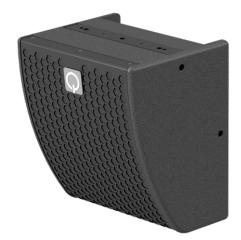
MODEL type filter power handling AES program power impedance sensitivity program SPL frequency range dispersion weight size (wxhxd) C6 6"ND/1"ND Coaxial passive 200W 400W 16 Ohms 95dB 118dB 60-20000Hz 80° nominal 8 kg 236x270x198mm
